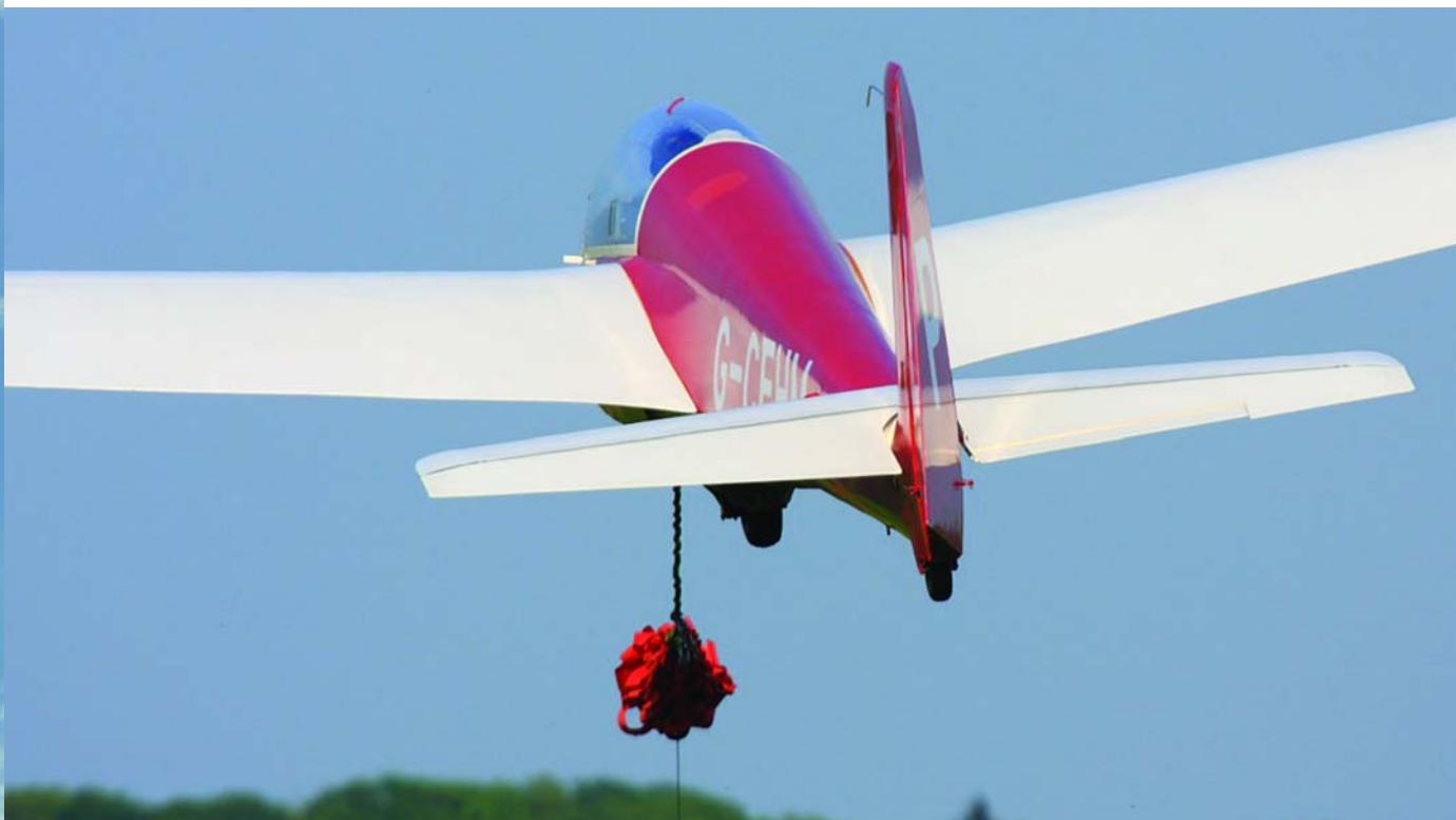
If a stall occurs during rotation it will be a dynamic or high speed stall after which the glider may flick roll. The glider is spinning while attached to the cable. The rolling of the flick roll is the autorotation of a spin. In some cases the glider hits the ground inverted with the cable still attached. Once the glider has stalled, recovery is probably impossible. You must anticipate and pre-empt this hazard.
